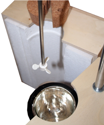
Dewar flask housed in insulated box and stirrer
