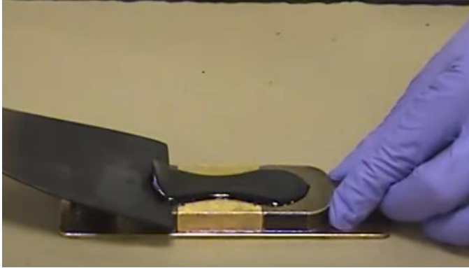
Figure 3: Cutting off excess bitumen
